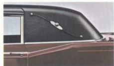
A rear seat control panel permits adjustment of radio and heater. Flow of cool air in the Seventy-Five's unique optional air-conditioning system may also be controlled by use of rear seat dials.
