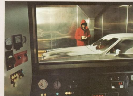
Effectiveness of Eldorado's new side window defoggers observed in Cadillac's Cold Room.
