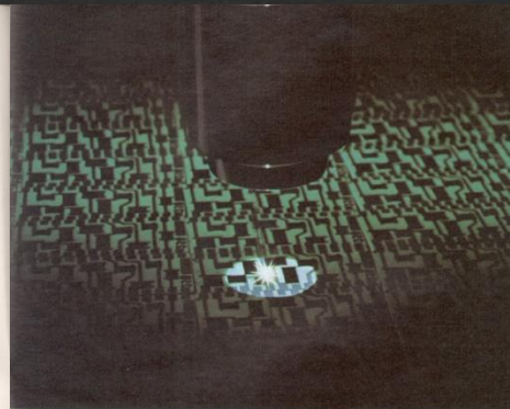
Laser trimming of Electronic Control Unit for Cadillac's exclusive Electronic-Fuel-Injected Engines.
