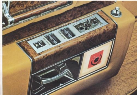
Power Control Panel on Driver's Door Armrest.
