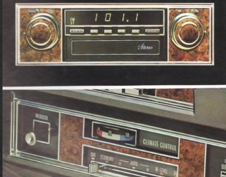
New Electronically Tuned AM/FM Stereo Radio with Signal Seeker, Scanner and Digital Display.
