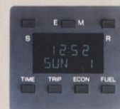
TRIPMINDER* COMPUTER. High-technology option offers you, at the push of a button, information such as the time, day, and date; trip odometer, trip average speed; instantaneous fuel economy data, trip average fuel economy, and fuel used.
