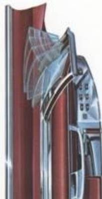
This view from above shows the driver's door console which houses controls for the six electric window mechanisms (wing vents are power operated, too), the master lock-out switch for them, and the power door lock* control.
