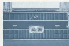
AIR CIRCULATION BOOSTER in rear door has powerful fan. Adjustable louvers distribute cooled or heated air.
