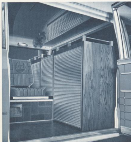
DELUXE DISPENSARY CABINET (this model, optional, extra) adds tremendous storage space. All sections of cabinet have M-M's aluminum space-saver Rol-Doors that slide open without protruding to hamper the movements of attendants. Standard set-up has two attendants' seats, with Tu-Way front seat that can be quickly changed from rear-facing to side-facing position (see page 5).
