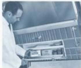
FIRST AID BAR in rear door expedites emergency care of patients outside the ambulance.
