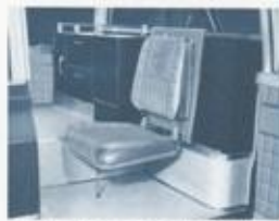
M-M's exclusive new Tu-Way Front Attendant's Seat (standard) is cleverly designed to face rear door (left photo) or side door (right photo) for greatest convenience in caring for patients. The seat
