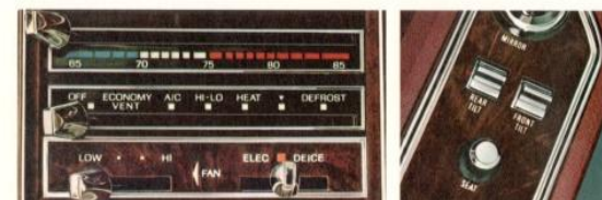
Automatic Temperature Control air conditioning with driver controlled fan speed.
