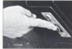
Cut-off switch shuts down entire electrical system. Protects against tampering.
