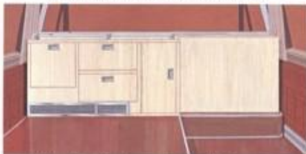
Storage for two D or E oxygen cylinders, at left. Two center compartments can have drawers instead of doors.
