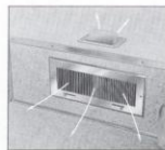
Heated air is dispersed by adjustable grille and deflector at stepwell.
