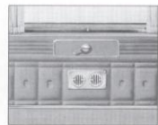
Air circulation booster fan, in rear door, has adjustable louvers.
