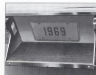
Lighted bumper step, with rubber tread, adds safety, convenience.
