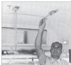
Insta-Ready Stretcher Hooks fold into overhead sleeves.
