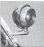
Spotlight/warning light reversible for clear or red lens.
