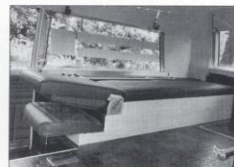
When lowered, jump seat back becomes adjustable head of bunk.
