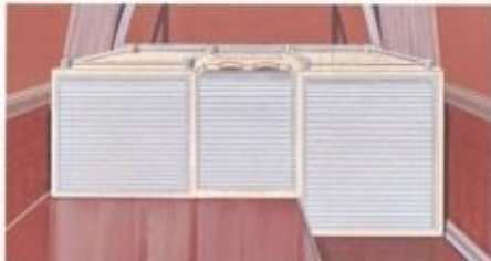
Storage for two D or E oxygen cylinders, at left. Two center compartments can have drawers instead of doors.
