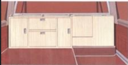
Standard cabinet (except Formica finish) has 5 compartments. Right compartment is for D or E size oxygen cylinders.
