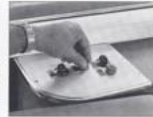
Switch panel on R.H. wheelhouse controls dome lights, rear heating system and other accessories.
