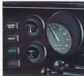
8000 RPM tachometer and Turbo indicator lights
