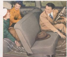
Tailor the weather to your measure with Studebaker's Climatizer. The new thermostatic control keeps a constant supply of warmed fresh air at an even temperature during cold weather. Separate quick-acting defroster. The Climatizer is available in all models at extra cost.
