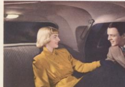
Automatic dome and map lights flash on when rear or front doors are opened. Lights may also be controlled from inside.
