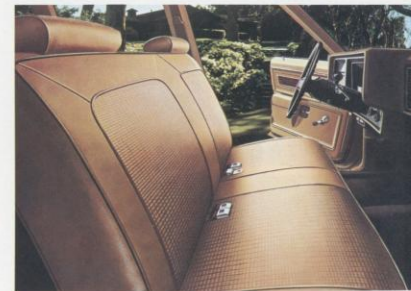
Deluxe interior. Deluxe wagons offer two all-vinyl interior choices: black or saddle. Doors are trimmed in matching vinyl; cargo area sidewalls are vinyl-coated metal. New molded full foam seat construction. Floor covering is color-keyed vinyl-coated rubber.
