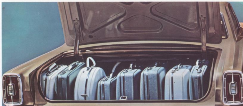
Big Fairlane trunk has 15 cubic feet of usable luggage space. Sill is lowered to bumper level for easier loading and unloading.
