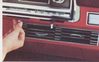
SELECTAIRE CONDITIONER: Air-conditioning, heating, defrosting are conveniently operated through a single control. Reheat feature removes moisture while cooling air.
