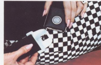
DELUXE SEAT BELTS: Automatic retractor reels outside front belts in to seat side. Seat belt reminder light flashes red on instrument panel.
