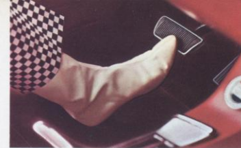
POWER BRAKES: Vacuum-assisted hydraulic type. Cuts braking effort by 55%. Wide, low pedal with short travel affords fast braking response for greater safety.
