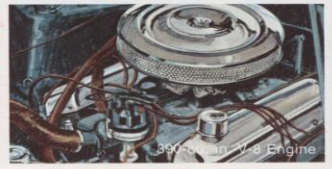
390-cu. in. optional Thunderbird Special V-8 Engine
