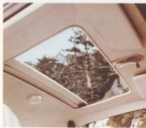
Manually-operated sun roof.
