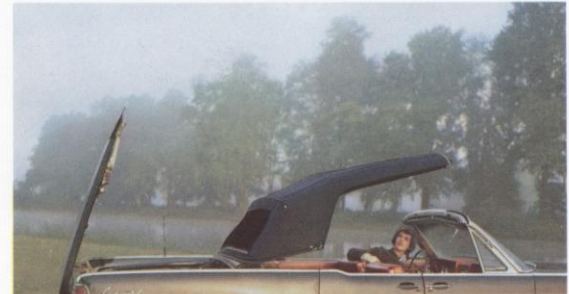
The weather-resistant top stores completely within the rear deck. When the top is raised, power locks secure it to the windshield, automatically.
