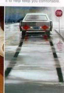
Track Master. This computerized skid-control system automatically pumps your brakes and maintains rear-wheel rotation for improved control during severe braking situations.
