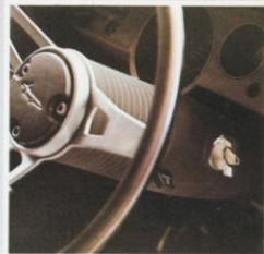
Anti-theft, column-mounted ignition switch.
