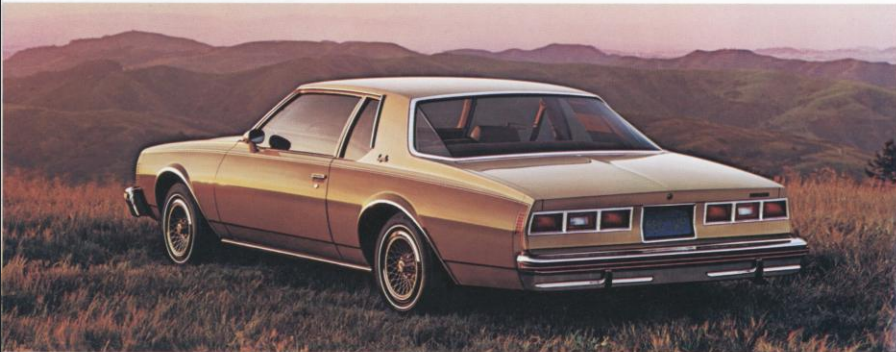
Impala Sport Coupe shown in available Custom Two-Tone beige and camel metallic with available sport mirrors, wheel opening moldings, sport wheel covers, white-stripe tires, bumper rub strips and bumper guards.
