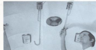
Insta-Ready Stretcher Hooks in roof fold into overhead sleeves. Optional, extra.
