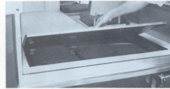
Convenient under-floor compartment at rear doorway stores two large stretchers. Standard on Cotington 54.
