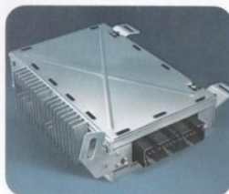
On-board computer for the Cadillac Electronic-Fuel-Injected Engine.
