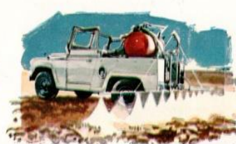
Numerous types of crop sprayers are available, the one shown here being driven from a pulley on the centre power take-off. Other types that can be driven from the rear power take-off are also obtainable.
