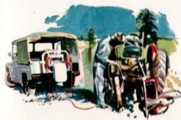
For the large farm or industrial undertaking—a mobile electric welding plant! Repairs can be dealt with immediately—on the spot—with this go-anywhere equipment installed in the vehicle and driven by the rear power take-off.
