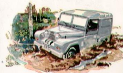
Another front mounted power take-off application is the drum winch—invaluable when traversing territory that's rougher than rough! The cable has a maximum pull of 2,500 lb.—sufficient for a Gipsy to haul itself up a near-vertical surface!
