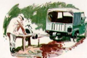
Another interesting job for the Gipsy! Using a drum type pulley driven by the rear power take-off, manual labour is considerably reduced with this stationary saw bench. Portable saws are available for attachment to the Gipsy where mobility is the first consideration.
