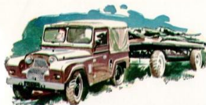
Many are the types of trailer that can be towed by the Gipsy. With four-wheel drive engaged, it has a maximum draw-bar pull of 4,000 lb., sufficient to tow a heavy trailer over really rough, or heavy, ground.
