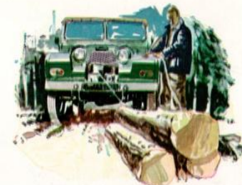
A front-mounted capstan winch has numerous applications, particularly among forestry undertakings.
