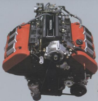
The heart of the NSX: the hand-built, all-aluminium V6 VTEC
