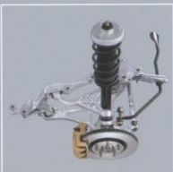
Independent double-wishbone suspension configuration comes straight from F1
