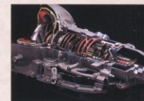
The fourth gear on Mark VII's automatic overdrive transmission is 100% mechanical drive, so there's virtually no slippage.
