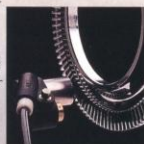
Mark's Anti-lock Brake System begins with a speed sensor at each wheel that sends information to a microprocessor.
