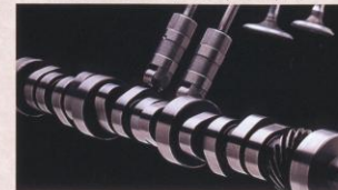
One example of applied racing technology is low friction roller tappets.
