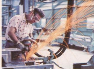
Careful welding of bodies is inspected at many points.
