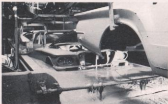
Bodies are actually immersed seven times for special cleaning, rinsing, and rustproofing treatments after welding.
