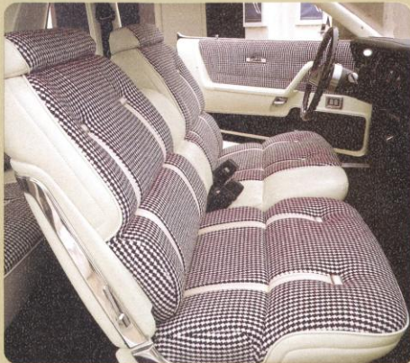
Optional Checkmate cloth with vinyl accents. 60/40 split-bench seat, folding center armrest, and dual reclining seat-backs with position controls.
