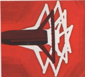
Tilt-a-Scope Steering Wheel telescopes 2.7 inches . . . tilts to five different positions.
