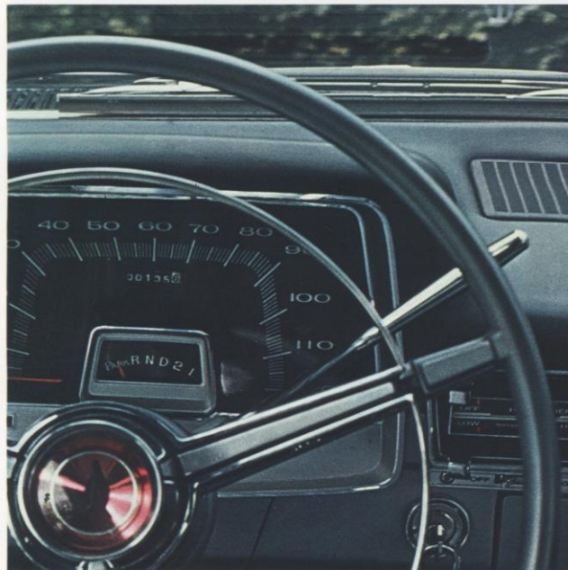
Automatic TorqueFlite transmission lets gears shift easily, conveniently, with a steering-column-mounted selector lever. (Indicator is mounted in the lower portion of the speedometer cluster.)
