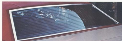
Electric rear window defroster with heating elements bonded to glass.
