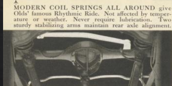
LATERAL STABILIZER BAR. One end anchored to frame and the other to rear axle. Prevents side-to-side movement and keeps frame and rear axle in alignment.
