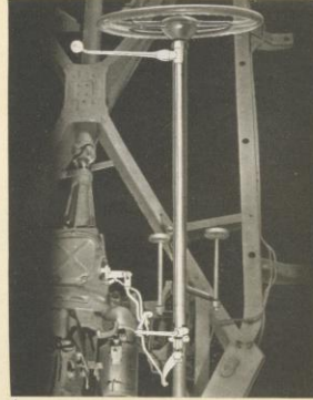
HANDI-SHIFT GEAR CONTROL greatly simplifies driving. The small lever just below the steering wheel is easy and convenient to operate.
