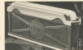
UNDER-HOOD, AIR-COOLED BATTERY. Oldsmobile batteries are of unusually sturdy construction. Locating the battery under the hood makes servicing easier and permits the use of short, more efficient lead wires to starter and generator. Air cooling lowers battery temperature.
