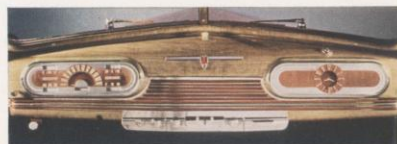
De Luxe Instrument Panel in Series 66 and 68. Instruments are grouped directly in front of the driver. A light in the glove compartment flashes on automatically when door is opened.
