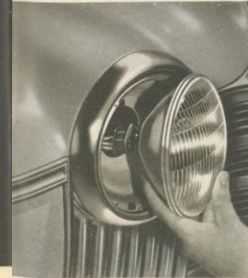
SEALED-BEAM HEADLAMPS. Lens is sealed to the reflector, preventing dust and water from reaching reflector surface.
