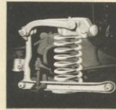
DOUBLE-ACTION HYDRAULIC SHOCK ABSORBERS. Proved cam and lever design. They control vertical motion, absorb road shocks, and take up rebound.
