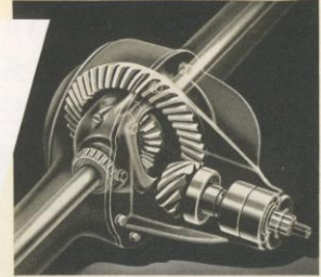
7-BEARING HYPOID REAR AXLE. Oldsmobile's rear axles are the semi-floating type, with power applied through hypoid gears. The center line of the pinion gear is below the center line of the ring gear, reducing bearing loads and resulting in quieter operation. The ring gear is bolted to the differential case to provide greater strength and rigidity. The use of seven anti-friction bearings cuts down rolling resistance, thus adding to long life.
