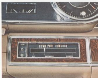
COMFORT CONTROL. Combines heating and air conditioning in a single unit. A dial permits setting of interior temperature as easily as with a home thermostat. Once set, the temperature is automatically maintained regardless of changes in the weather or the season.
