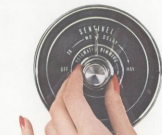
CRUISE CONTROL. Permits dialing of desired speed. Cruise Control is entirely disengaged by turning off ignition or manual "off" switch. It can be temporarily disengaged by touching the brake pedal. A new ruby colored light indicates when the system is in automatic operation and a new lighted dial illuminates the numerals.
