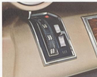
CRUISE CONTROL. Permits dialing of desired speed. Cruise Control is entirely disengaged by turning off ignition or manual "off" switch. It can be temporarily disengaged by touching the brake pedal. A new ruby colored light indicates when the system is in automatic operation and a new lighted dial illuminates the numerals.
