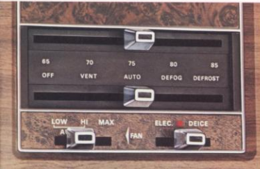
Automatic temperature control
