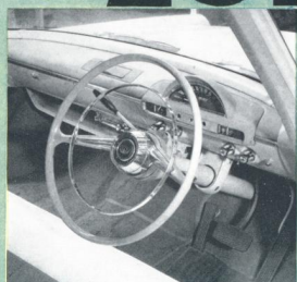
The Zodiac steering wheel with its full circle horn-ring through which the neatly grouped instruments can be clearly seen.
