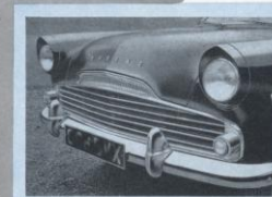
A styling feature is the modern treatment of the hooded headlights. Beneath these are separate parking lights which incorporate the front-turn signal lamps.
