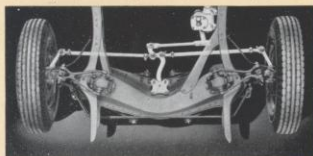
Knee-Action Wheels and Balanced Springing: Oldsmobile's Knee-Action Wheels "step over" humps and holes. Independent, free-acting coil-springs "float" you along with an easy, gliding ride.
