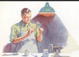
Rifle-Drilled Connecting Rods: Carry oil under pressure to piston pins, also drilled to spray cylinder walls, adding greatly to life of pistons, rings and cylinders. (Left)
