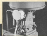
Automatic Choke Control: Eliminates over-choking or under-choking, promotes easy starting in cold weather, smoother operation during the warm-up period. (Above)
