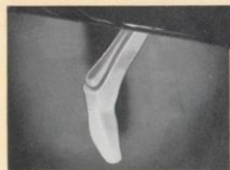
Hand Brake Lever: Conveniently and naturally located under the dash within easy reach of the driver's left hand.
