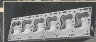
High Compression Cylinder Head: This efficient design permits a high combustion ratio for dashing performance and economy.
