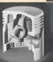
Electro-Hardened Aluminum Pistons: This type of construction reduces weight of reciprocating parts and helps lengthen the life of main and connecting rod bearings. Piston shape is maintained by top ribbing and reinforcement. (Above)
