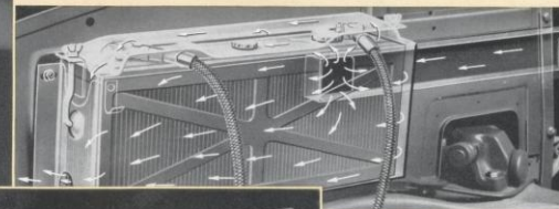
Under-Hood, Air-Cooled Battery: Located under the engine hood in an enclosed compartment making it accessible for service. A special duct assures circulation of cool air around the battery. (Above)
