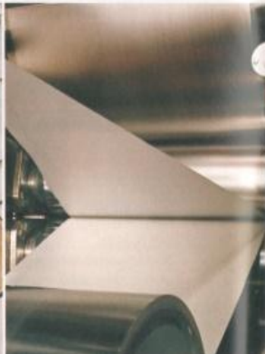
Manufacturing bi-metal moldings for corrosion protection.
