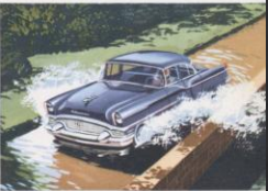
SENDING twin sprays flying, a Clipper sweeps through the water bath. This thoroughly tests chassis, engine and electrical system for waterproof qualities.
