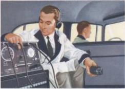
HERE is how disturbing noise is farthest out and its origin determined. This instrument scientifically records the sound level in every section of the car's interior.
