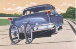
THE INSTRUMENTS mounted on the "bicycle wheel" carriage measure speed and acceleration with utmost accuracy on the world's fastest 2 1/2 mile closed track.
