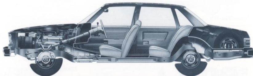
Full-Perimeter Frame • Full Coil Spring Suspension • Adult-Size Head Room and Leg Room • Shown with optional police tires
